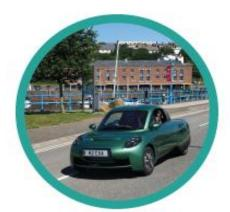
The Riversimple Rasa is an electric car powered by hydrogen rather than batteries. The hydrogen passes through a fuel cell, where it combines with oxygen from the air to produce electricity. This electricity flows to small, lightweight electric motors, one in each wheel, which give the car 4 wheel drive. The only emission is water.
